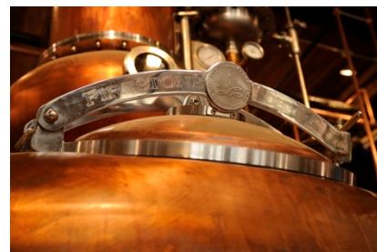
Two 500-gallon copper pot stills by Vendome Copper and Brass Works
